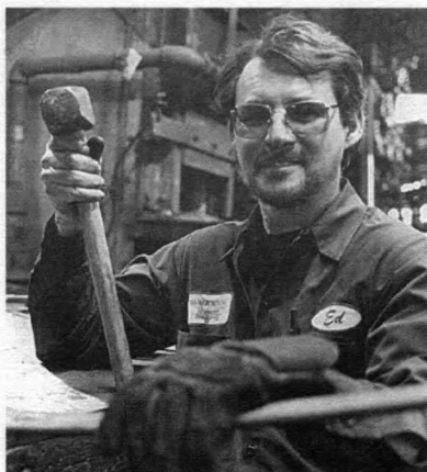
Blacksmith Ed Weidele poses with an eight-pound sledge hammer he uses to shape the steel after it comes out of the gas-fired furnace.
